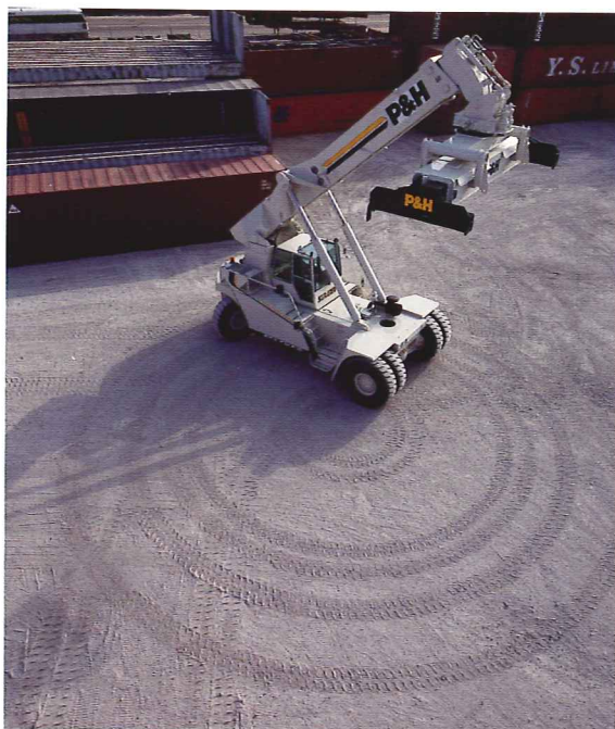
Tight turning radius of 26'3" means Superstacker works well in cramped quarters.
