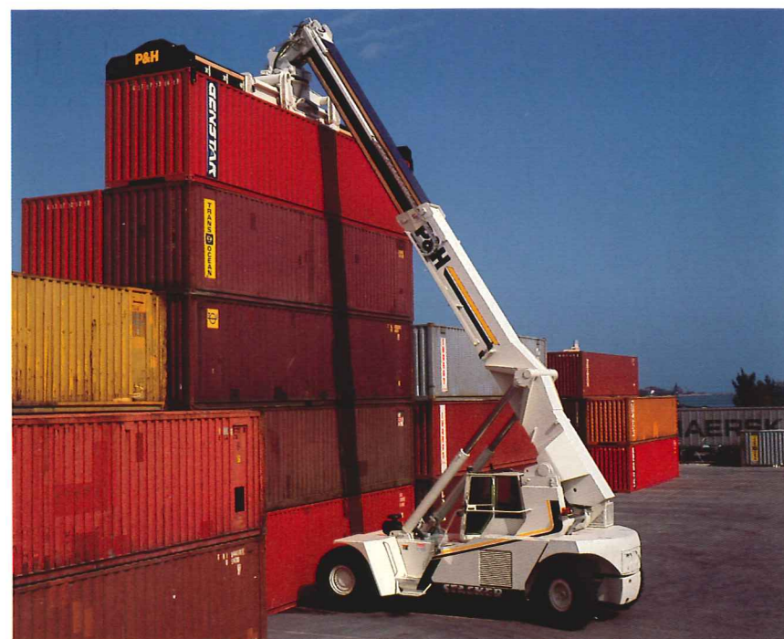
Superstacker makes it easier to stack 44-ton containers 4 or 5 high.
