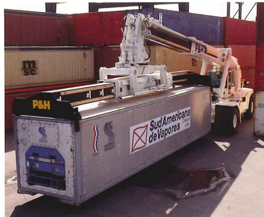
Telescopic boom and non-continuous 360° spreader swing allow 20' to 40' end-on container handling.
