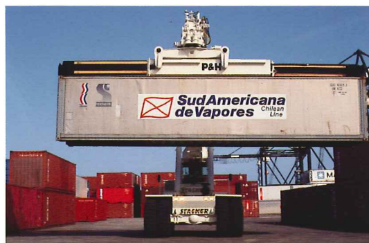
Superstacker compensates for unevenly distributed loads.
