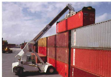
Twenty-four ton second row capacity gives Superstacker added flexibility. Superstacker handles third row weights of up to 9.5 tons.
