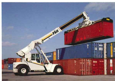
Thanks to Superstacker's extended reach, containers can be stacked 3 rows deep for more efficient use of your space.
