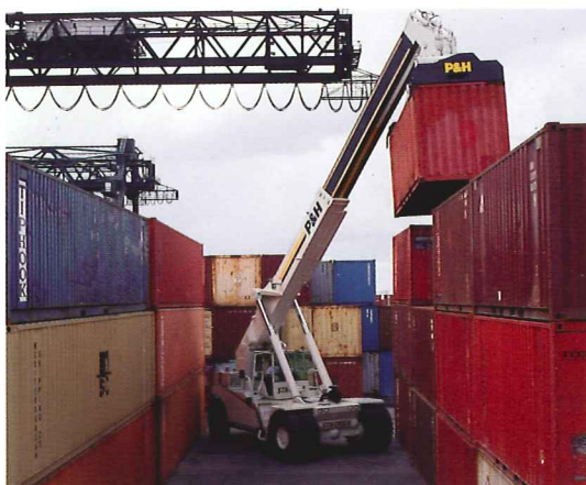
Flexible and accurate slewing allows Superstacker to handle containers in very tight places.
